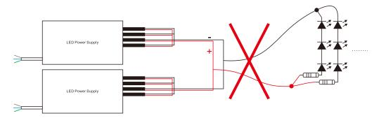
(2) It is allowed to use parallel connection for outputs from 1 power supply
