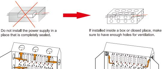
Perforate the sides of the metal case or use an eletric fan to make the heat release easily
