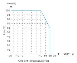
ambient 50°C → 80% of rated wattage ambient 60°C → 60% of rated wattage
